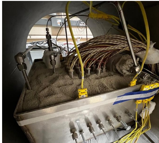
Instrumented and insulated test specimen
