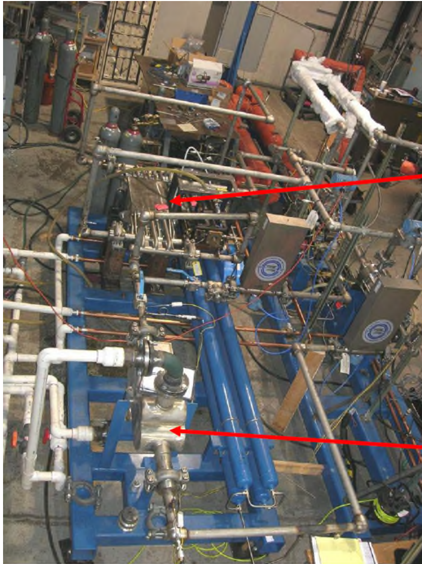
sCO 2 test loop used by Sandia/ Barber-Nicholls
