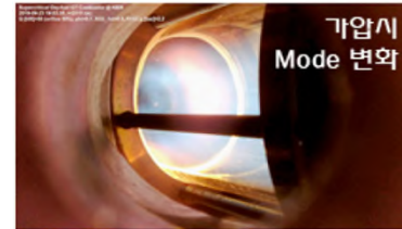
237 kW th , \phi=0.7 , X_{O_2,1st}=0.6 , F=20
