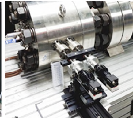
Design of 300 bar oxy-fuel combustor
