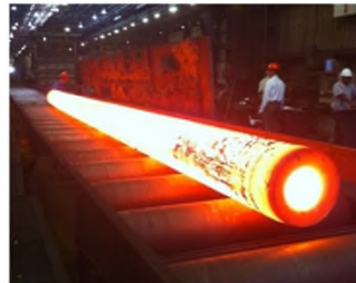
First 740H Pipe Extrusion
