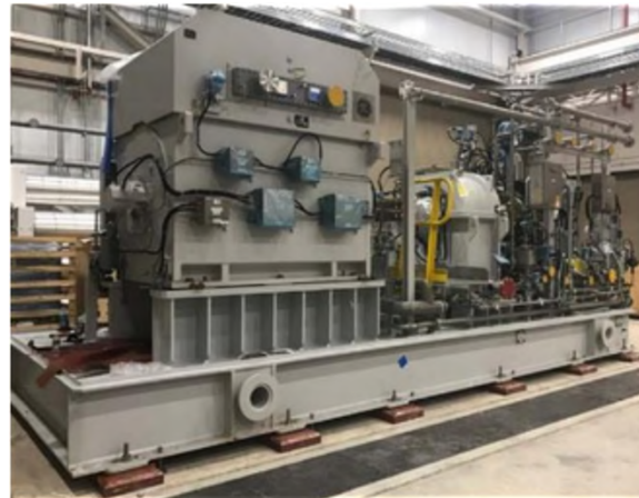
sCO 2 compressor skid [Stevenson, 2024]
