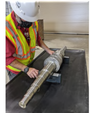
STEP Turbine Rotor (Monolithic Nimonic_105_rotor, EDMed)
