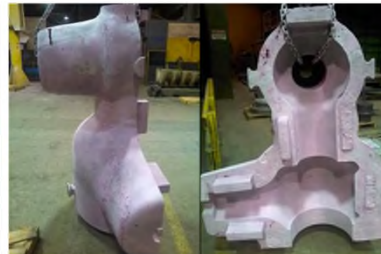
H282 Valve Body Casting (after PT)
