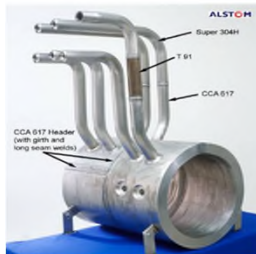
Header Welding Demonstration
