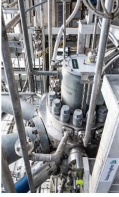
Compressor prototype installed on the test rig at the Baker Hughes facility in Florence, Italy
