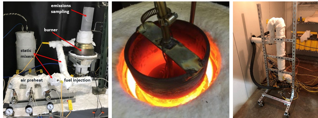
High-Temp. Recuperator (L), Porous Matrix Burner Development (C), Direct-fired Desorber Tests at -30°C (R)
