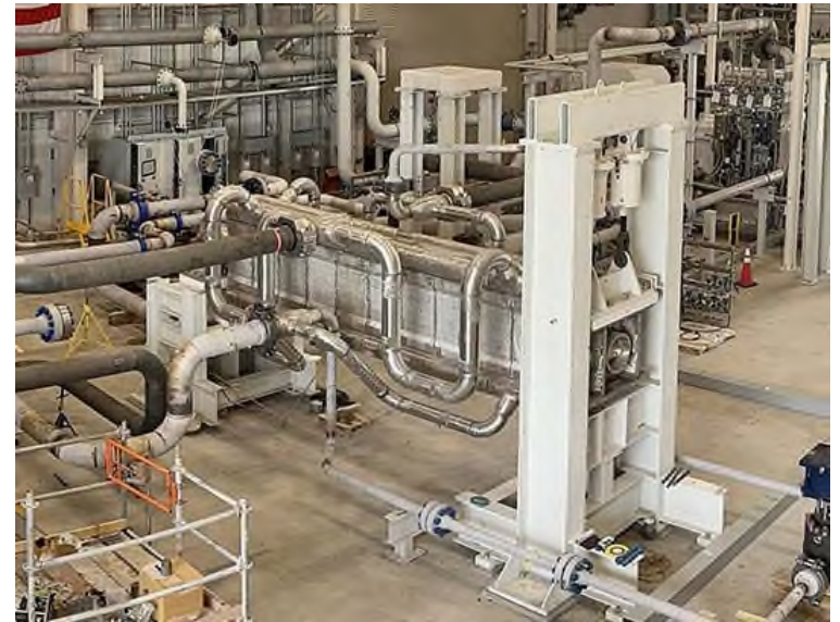
PCHE Recuperator for STEP program
