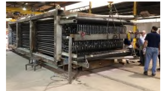
STEP 10 MWe Facility Natural Gas Fired Heater
