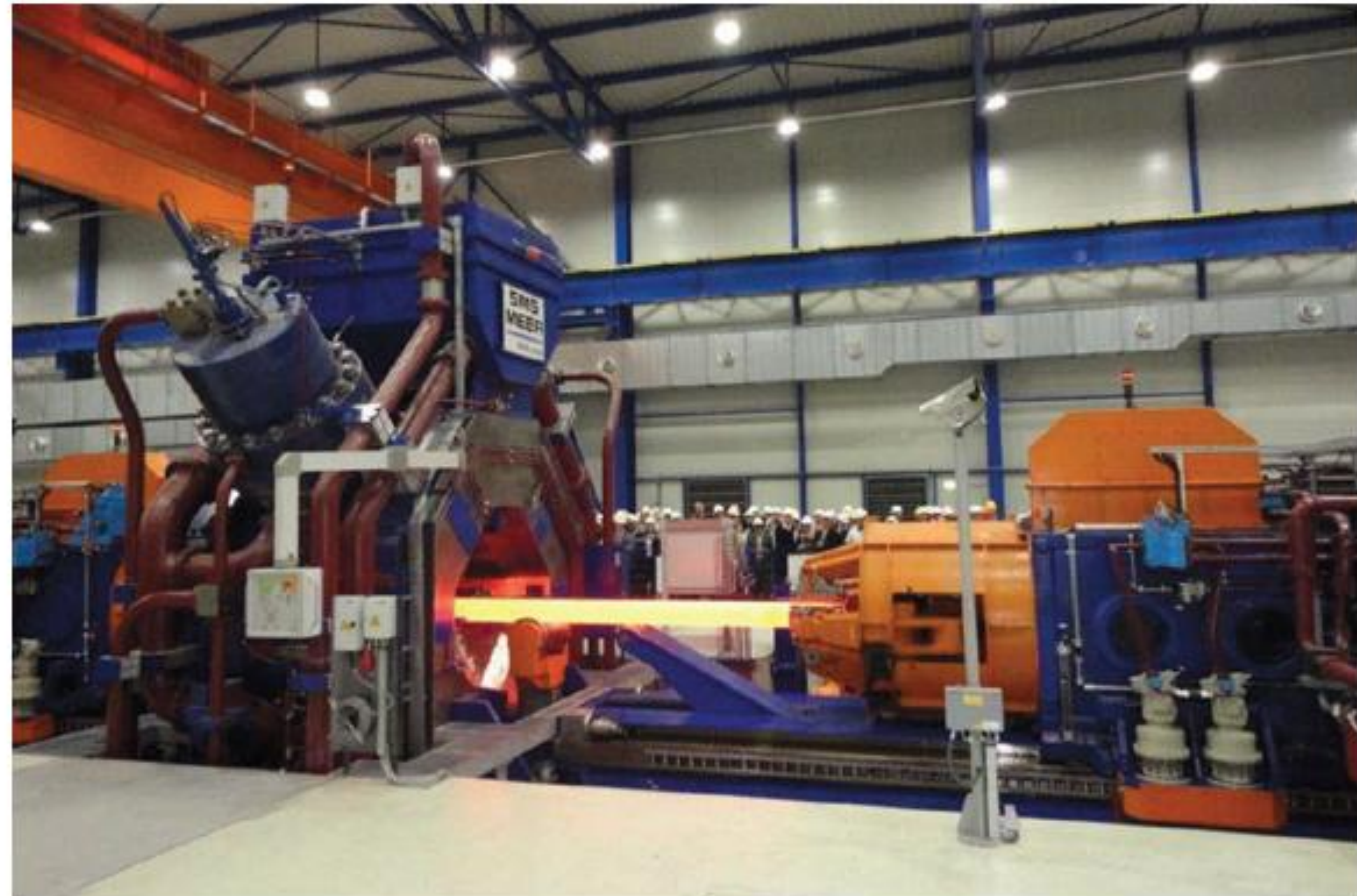
Radial Press SMX-800/25MN and rail bound manipulator
