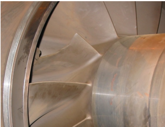
Impeller blade failure (Pettinato, et al., 2013*) Causes: Choke operation, liquids, resonant operation (?)
