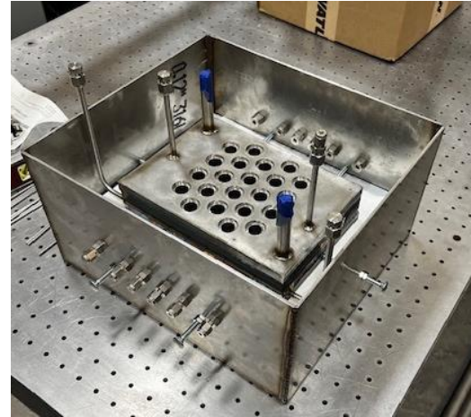
Test specimen insulation tray
