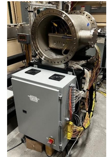
Heat exchanger test apparatus
