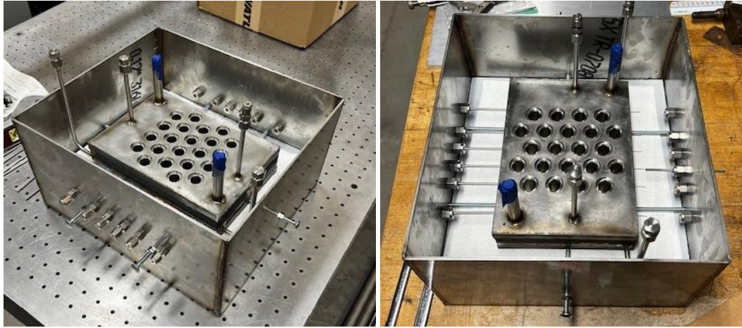
Figure 4. Test specimen positioned within the insulation tray after machining and installation of process connections.
