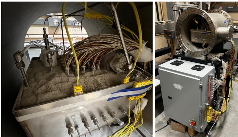
Figure 7. Insulated and instrumented test specimen and test apparatus.
