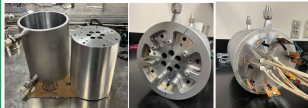
Assembly process of post-machined cold plate and heater column with heating elements and instrumentation.
