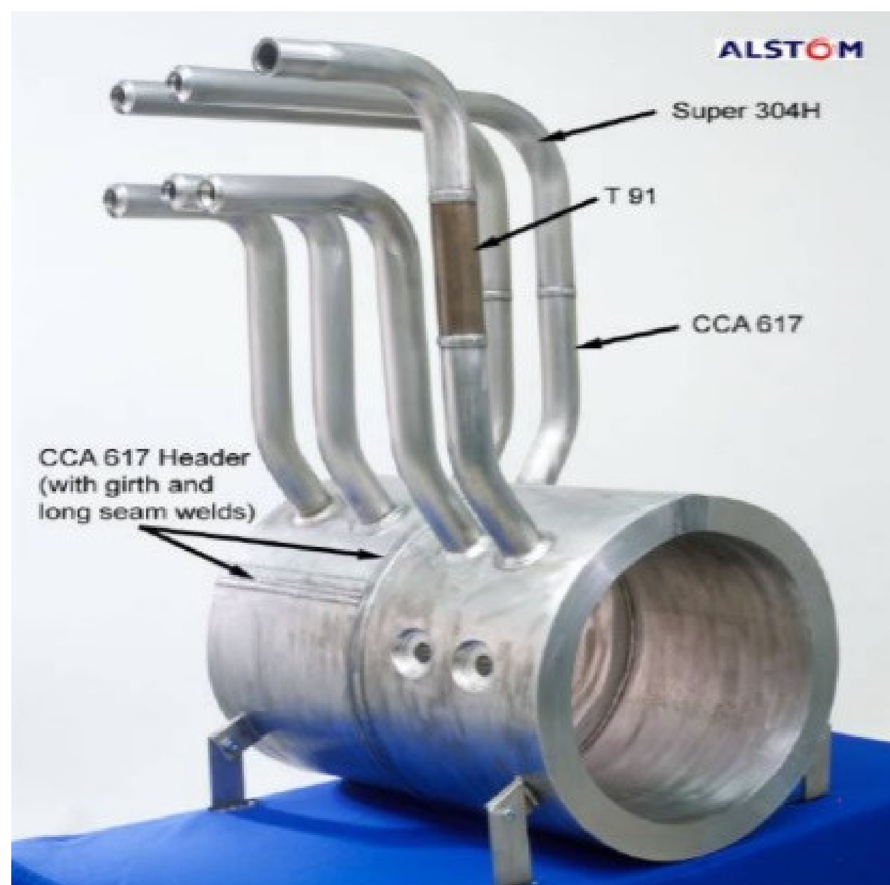
Header Welding Demonstration
