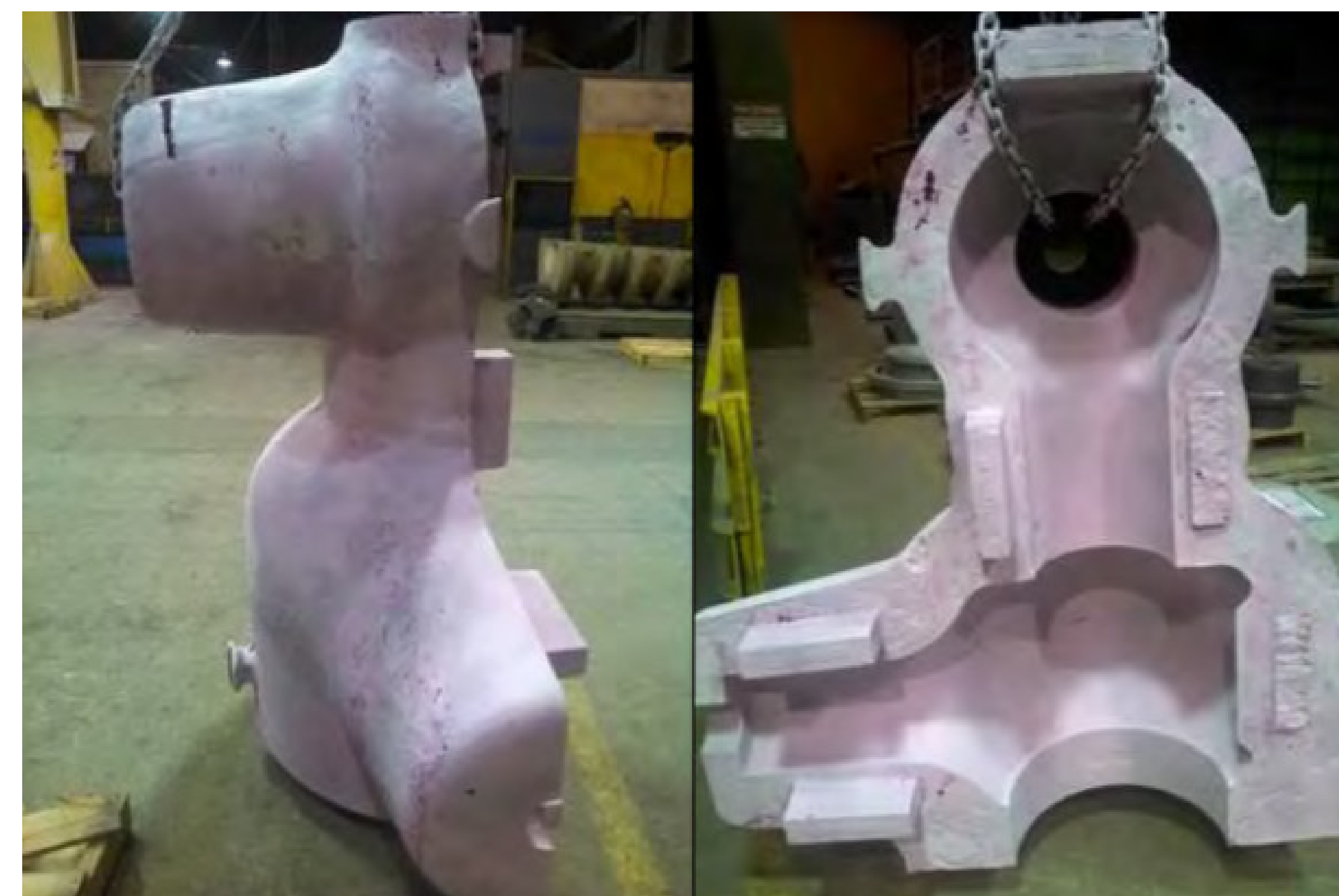
H282 Valve Body Casting (after PT)
