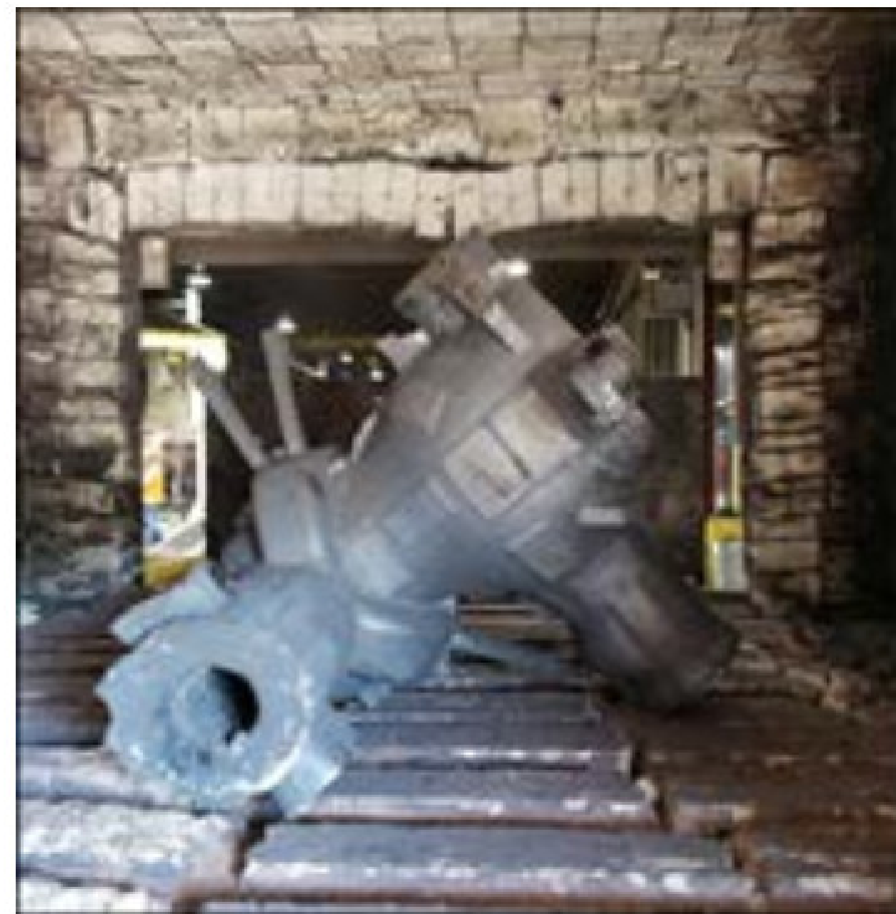
Turbine Stop Valve ( Haynes 282 ) Alternate valve from 316SS
