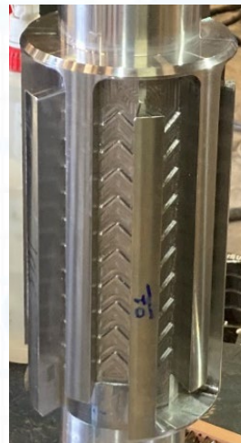
Internal Blade Cooling Heat Transfer Testing
