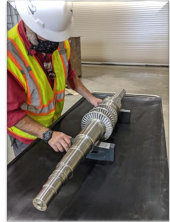
Figure 5. Rotor of STEP sCO 2 turbine
