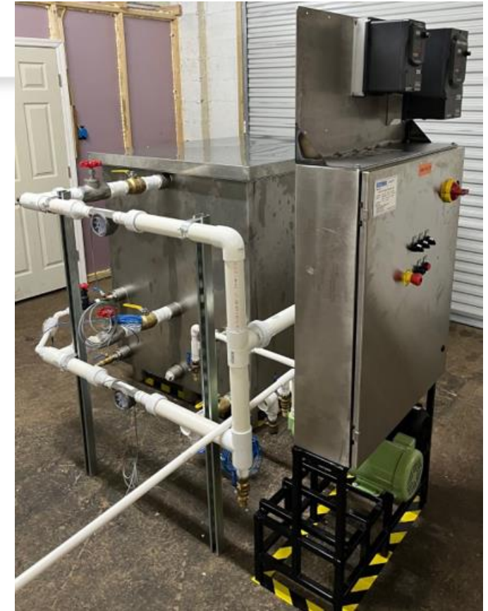
25kWth I 2 HEX testing at AES facility: (2023-2024 at AES; 2024 at Echogen)
