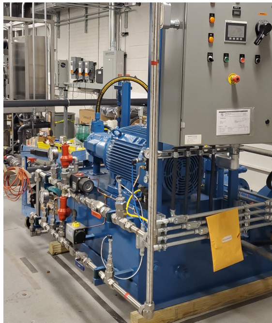
Figure 11: Laboratory-scale HPSG using low-speed reciprocating compressor.
