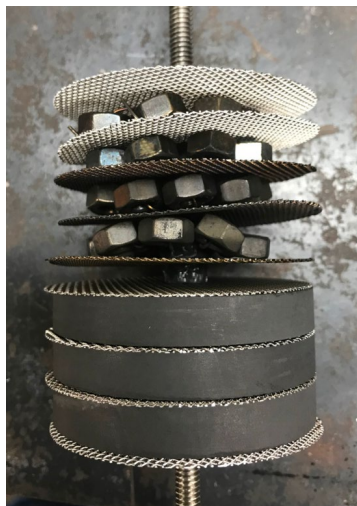
Figure 5. Photograph of four layers of stainless steel nuts (used as specimens mock-up) on top of three stacked 2.5" diameter graphite susceptors.
