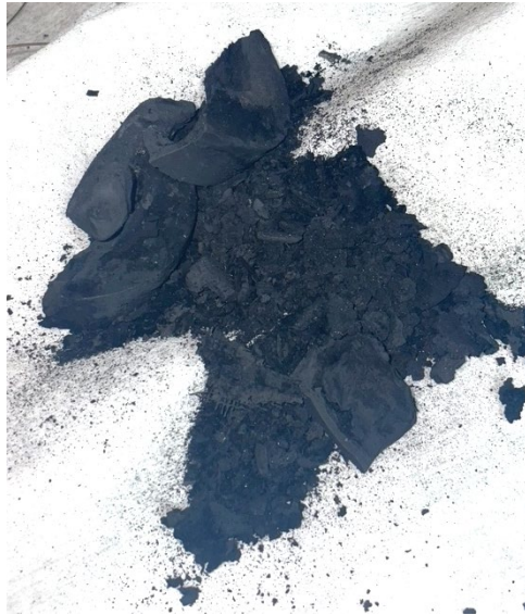
Figure 11. Failed graphite susceptor after high temperature exposure.
