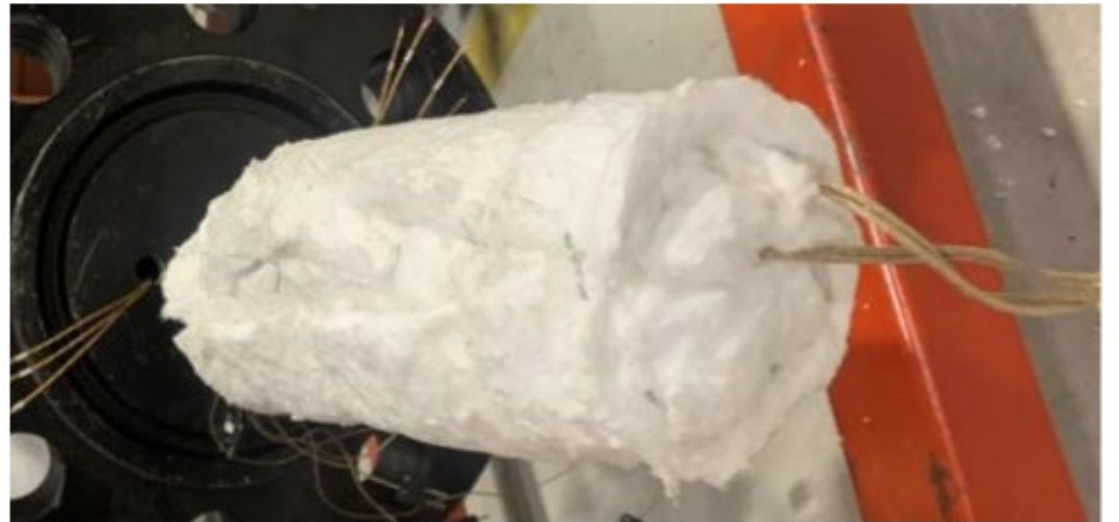
Plumbed and wrapped internal assembly
