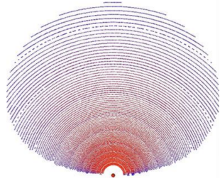
Figure 14: Sample heliostat field for one receiver. [53]
