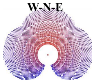
Figure 16: North, East and West facing three-receiver tower solar field simulation. [53]
