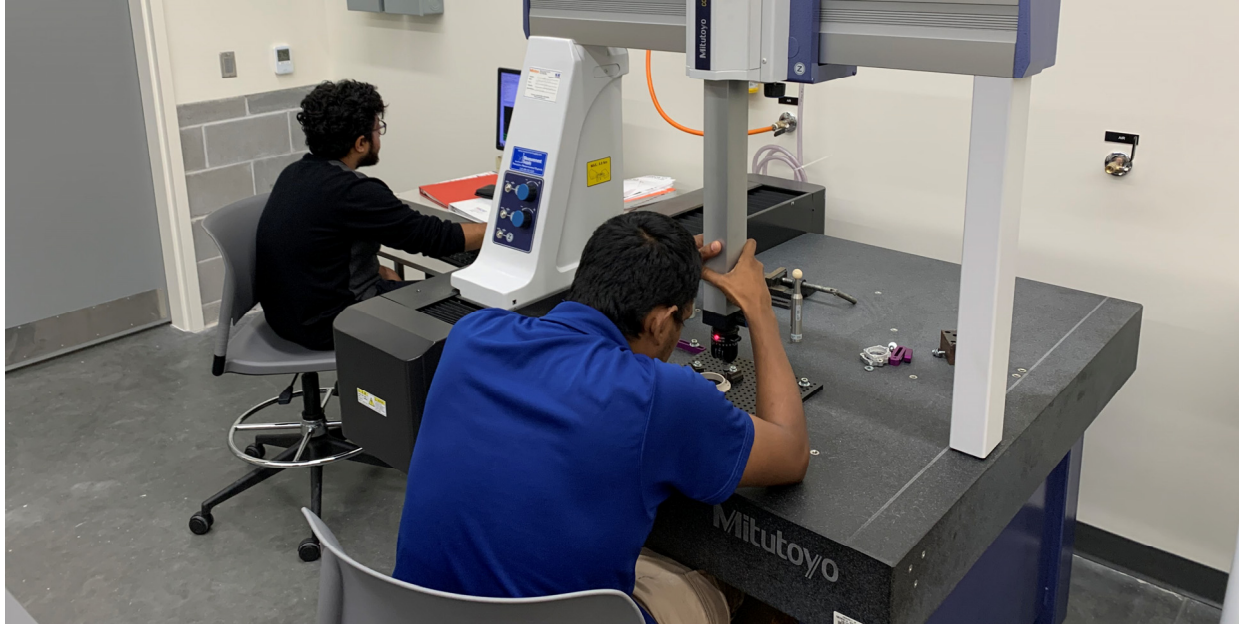
FIGURE 8: Seal dimensions measurement using CMM machine.
