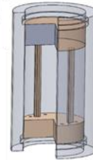
Figure 28: Buildup of a testing package for bearings. This example is for the testing of an active PM biased combination radial and axial bearing
