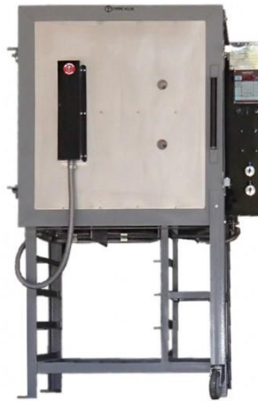
Figure 23: PMRMB test chamber Olympic FL10E radiant kiln furnace
