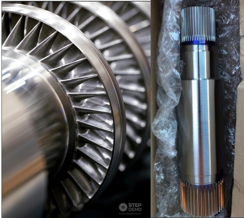
Figure 13 - Close up of EDM Turbine Blades along with Spline Test Piece
