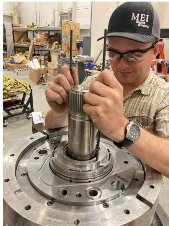
Figure 18 - Installation of Dry Gas Seal
