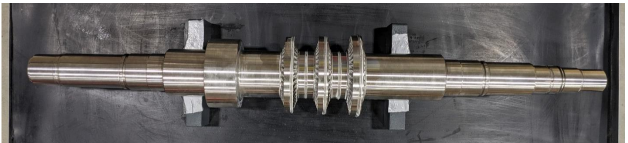
Figure 12 - Turbine rotor following rough machining and EDM
