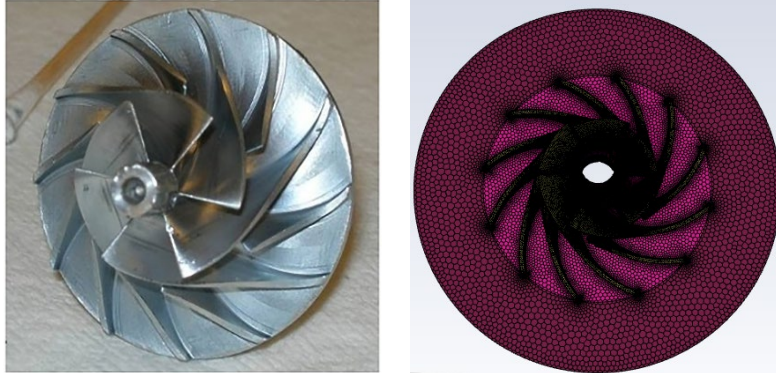
Fig.7 Geometry of Sandia impeller: (left) original prototype; (right) reconstructed impeller mesh
