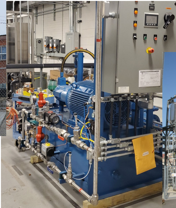
CO 2 heat pump & power cycle
