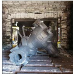
STEP turbine stop valve and body casting (Haynes 282)
