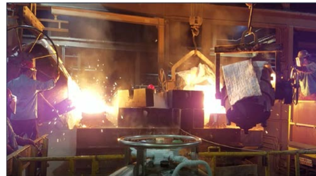
Haynes 282 casting for STEP TSV
