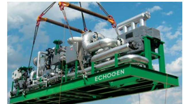
Compact arrangement example Echogen EPS100
