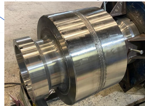
1-Piece Fabricated Inconel Casing
