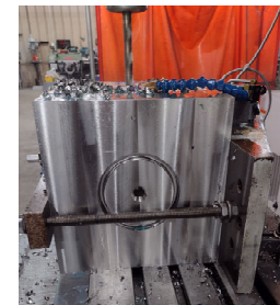
Heat transfer feature assembly with heater and instrumentation
