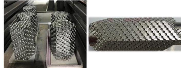
Printed, de-powdered, & sintered SS316L HX cores
