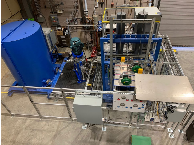
Supercritical CO 2 seals test rig 4,000 psi @700C 40,000 rpm • Shaft size of 10MWe system
