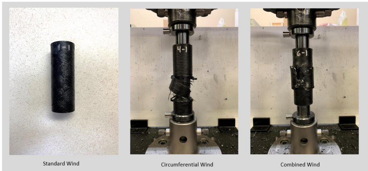
Figure 37. Failed Multilayer 1.25-inch OD Hoop Specimens 125NCG-4X21L (Helical/Standard Wind), 125NCG-4H21L (Circumferential/Hoop), and 125NCG-4C21L (Combined) – Left to Right.
