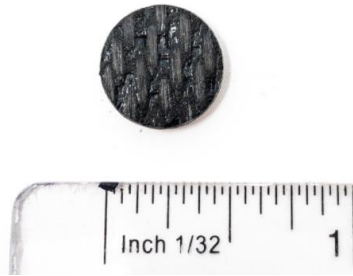
Figure 21. Thermal Conductivity Specimen (0.5” Diameter).
