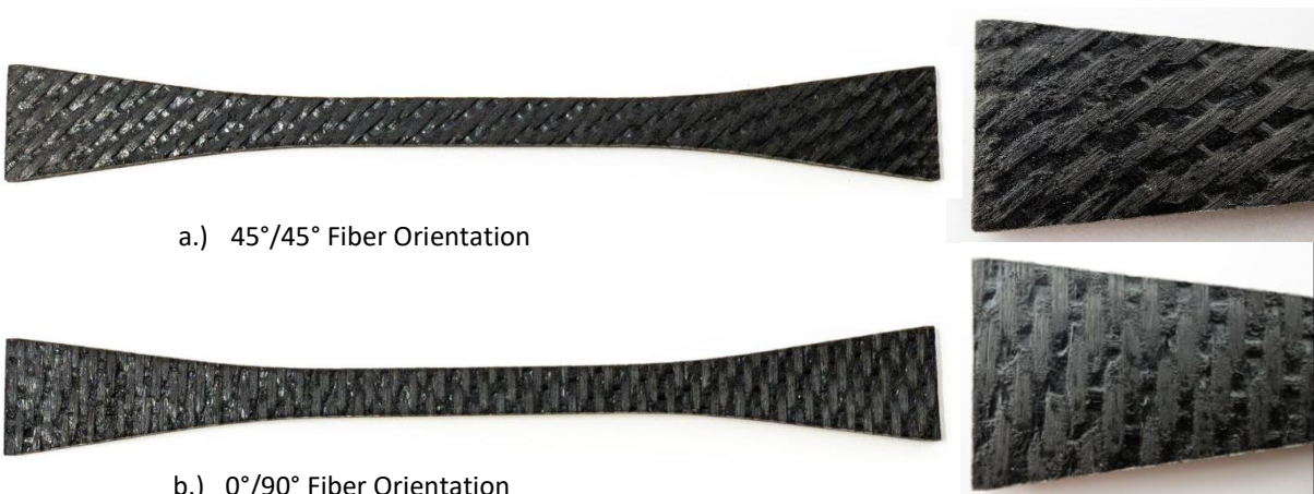
Figure 18. Tensile Test Specimen with 0°/90° and 45°/45° Fiber Orientations.
