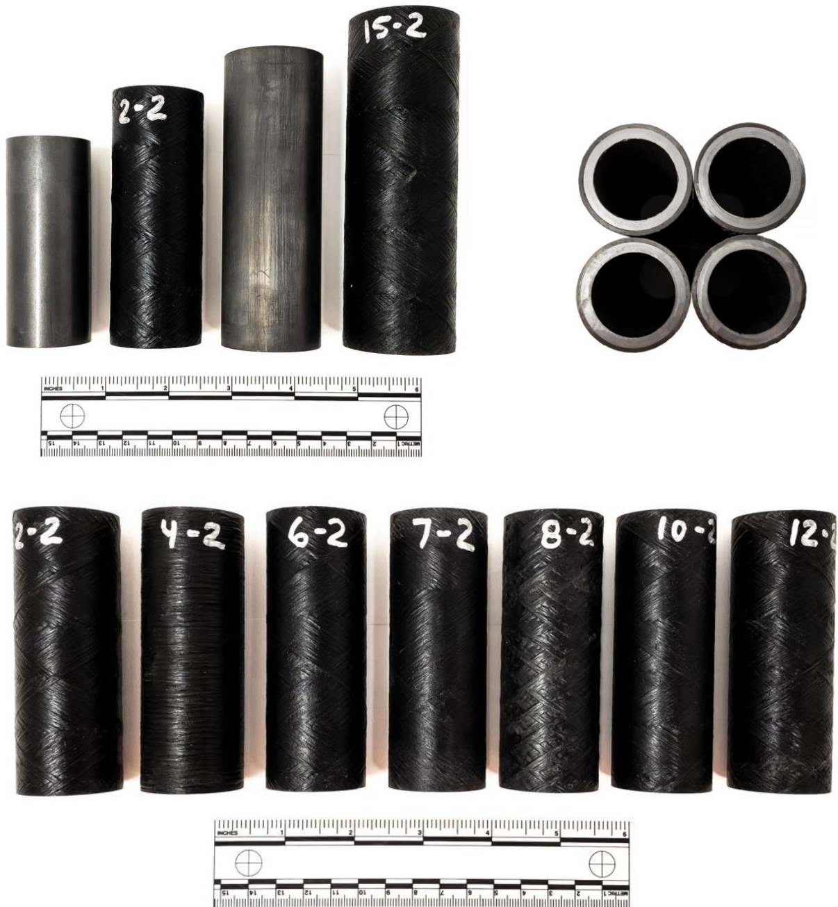
Figure 34. Top-down View of 125 HEXOLOY, 125NCG-4X21L, 150 HEXOLOY, and 150NCG-4X21L Hoop Test Samples – Left to Right (top left), Specimen Cross-section of 125 Multilayer Hoop Test Samples (top right), Top-down View of All Multilayer Hoop Test Sample Configurations – 125NCG-4X21L, 125NCG-4H21L, 125NCG-4C21L, 125NCG-4X11L, 125NCG-4X81L, 125NCG-4X21H, 125NCG-4X21L-ND – Left to Right (bottom).
