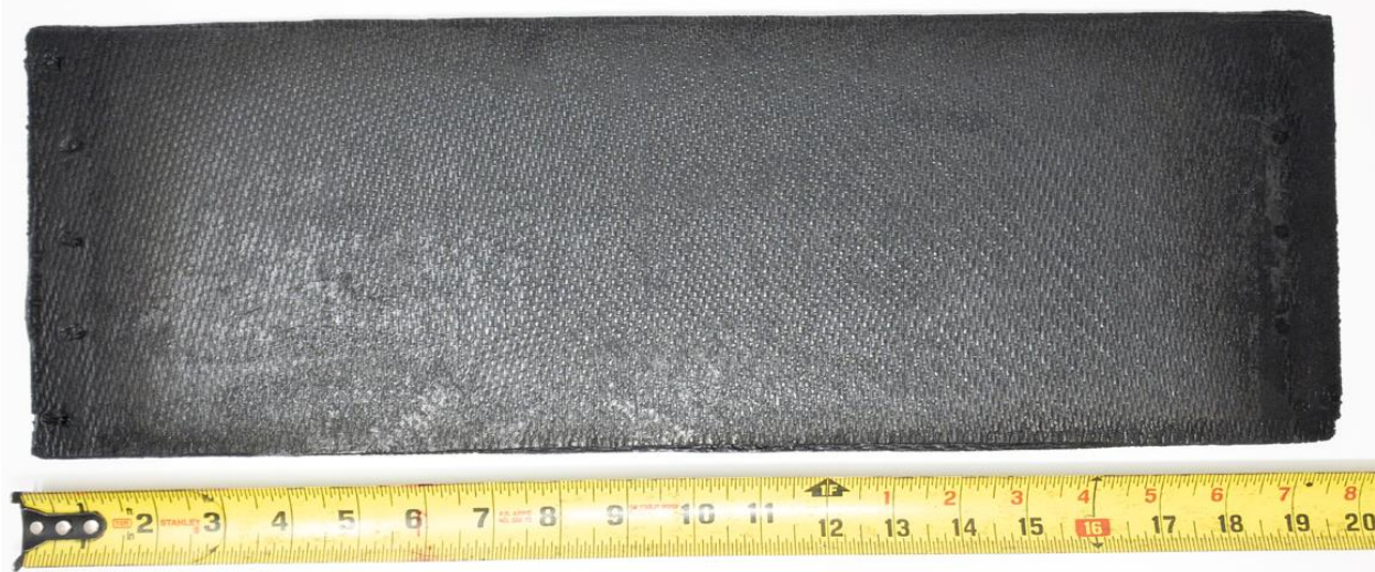
Figure 16. Densified SiOC i /SiOC Composite Plate.
