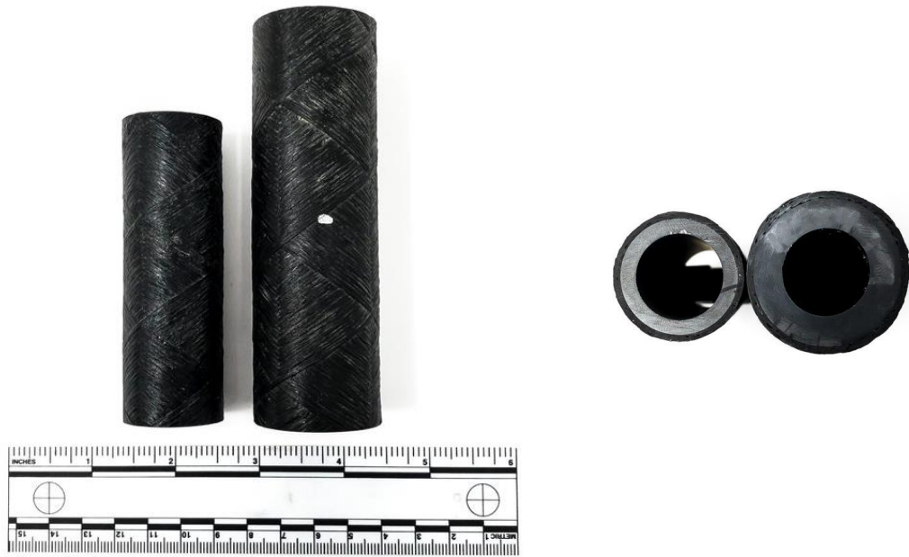
Figure 26. Top-down View of 100X4 and 125X4 Specimen (left) and Specimen Cross-section (right).
