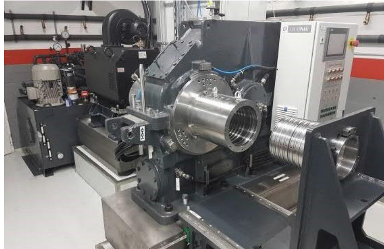
Picture 1: Tester setup / overall specification of the ultra-highspeed-tester
