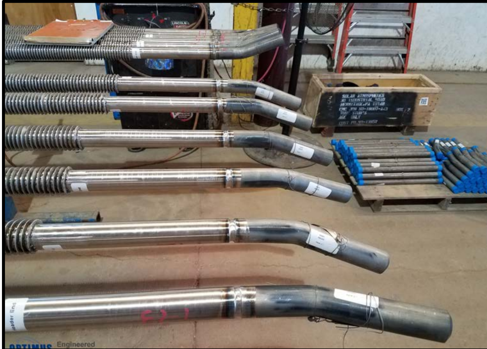
Welding of tube bends to straight sections of coiled tubing
