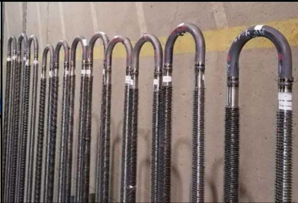
Welding of tube bends to straight sections of coiled tubing
