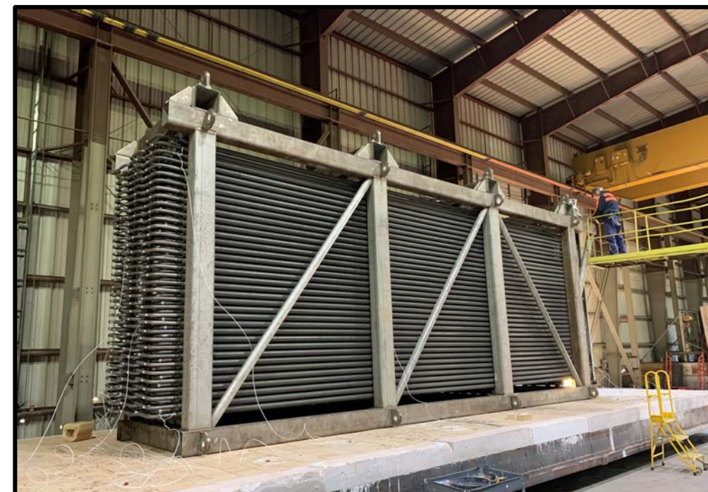
Coil Assembly in Frame Prior to Heat-Treatment
