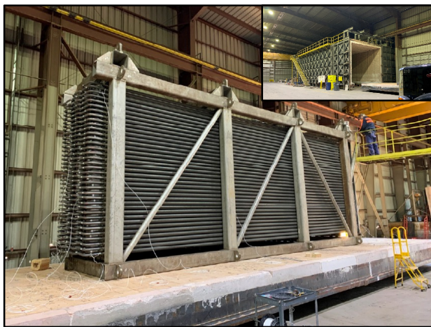
Figure 4. Heater coil prior to heat treatment (insert is picture of heat-treatment furnace)
