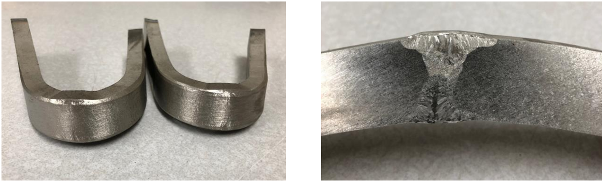
Figure 12. a) Side bend test bars, b) Weld cross-section
