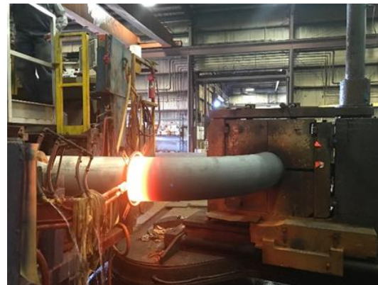
Figure 2. Induction bending of welded pipe
