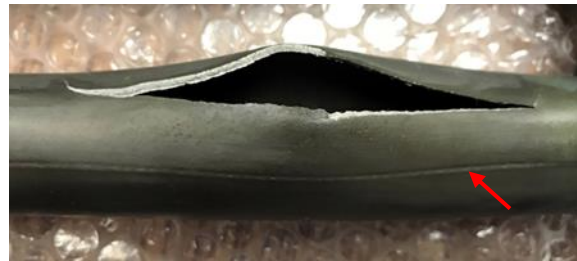
Figure 3. Burst test specimen. Location of the weld seam indicated by arrow.
