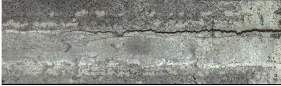
Figure 7. Tube OD view of fractured creep specimen
