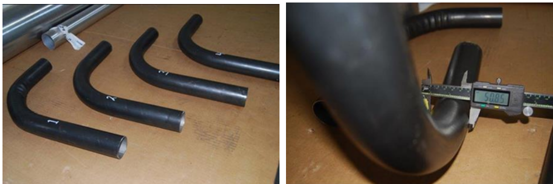
Figure 9. a) Bent tube samples, b) measurement fixture (Tibunas)
