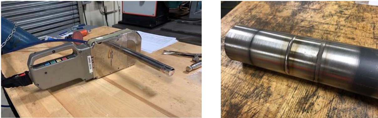
Figure 10. a) Welding head, b) Test specimen
