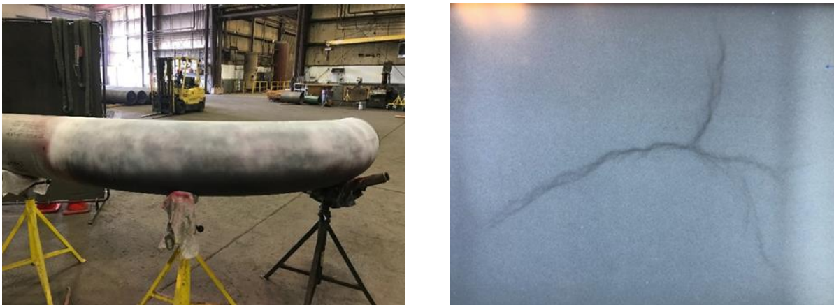
Figure 15. a) Completed pipe bend, b) radiographic image of ID crack.
