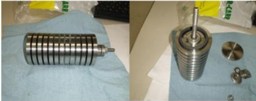
Compression fixtures designed to hold the O-rings inside the sCO 2 autoclave
