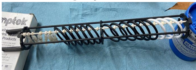
O-ring compression jig used in sCO 2 exposure; 25% deflection shim used
