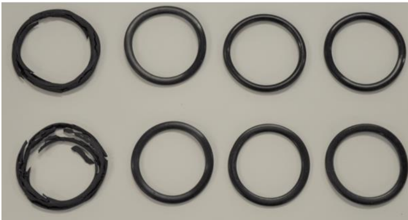
Picture of whole O-rings after compressed exposure to 20 MPa sCO 2 at 100°C: from left – top row: Viton sample 1, Buna N, EPDM, HNBR; bottom row – Viton sample 2, EPR, Neoprene (uncoated) and Neoprene (coated)
