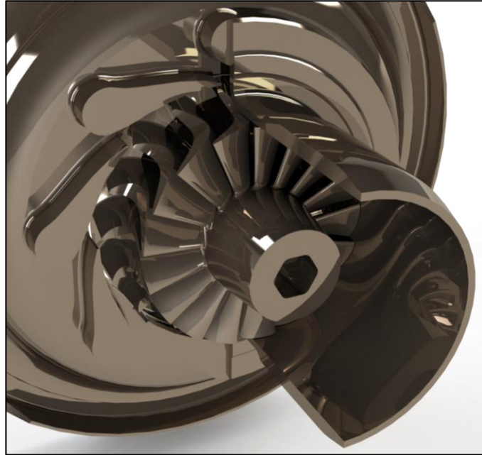
Figure 1: PTT 1MW turbopump development, HPT rotor, nozzle, and exhaust (sectioned).
