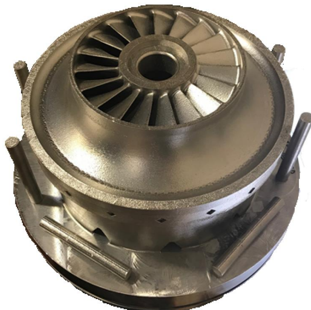
Figure 6 - Turbine Wheel and Test Coupons after Build
