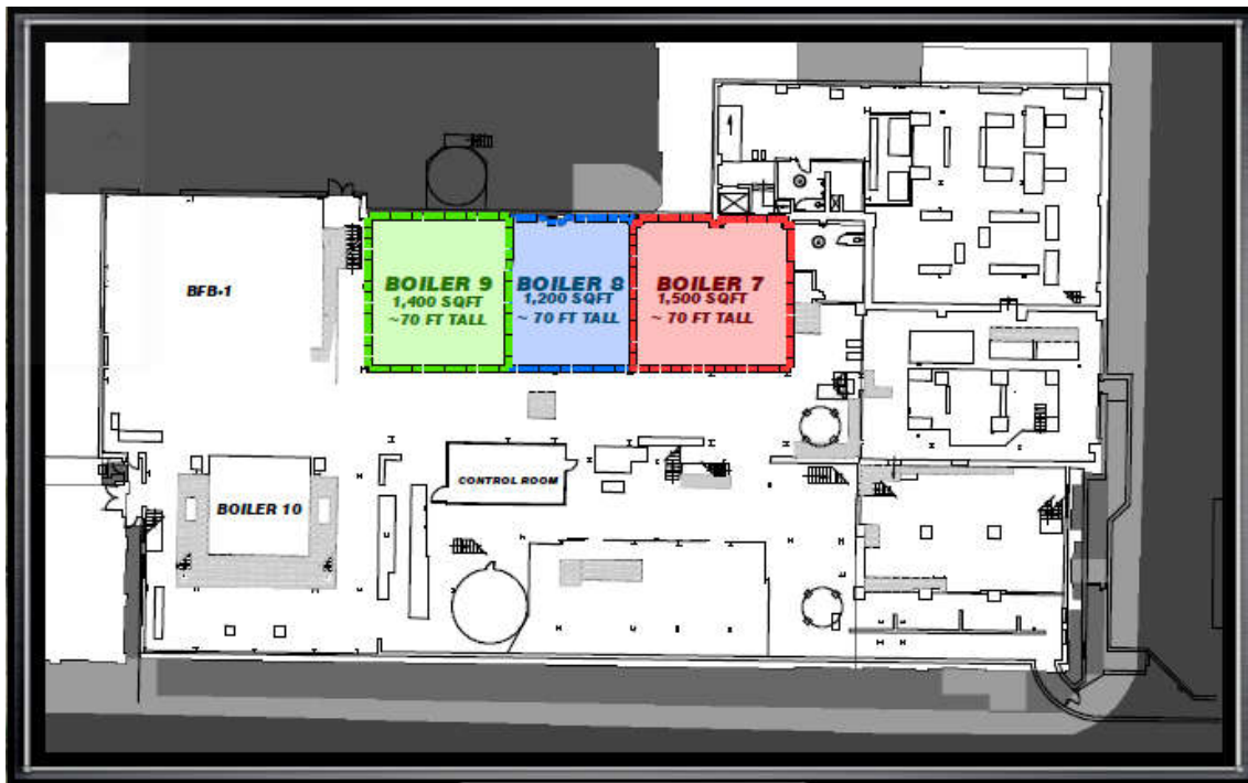
Figure 2 – MU CCHP existing boiler building layout, highlighting the units to be removed
