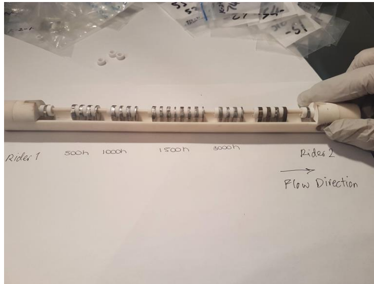
Figure 3: Test samples inside the alumina specimen boat prior to the first test.
