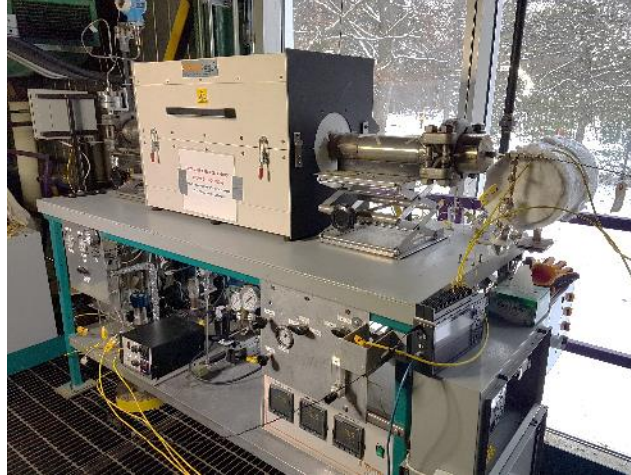
Figure 1: High pressure and temperature supercritical CO 2 corrosion test rig, jointly developed by Natural Resources Canada's CanmetENERGY-Ottawa and Carleton University.
