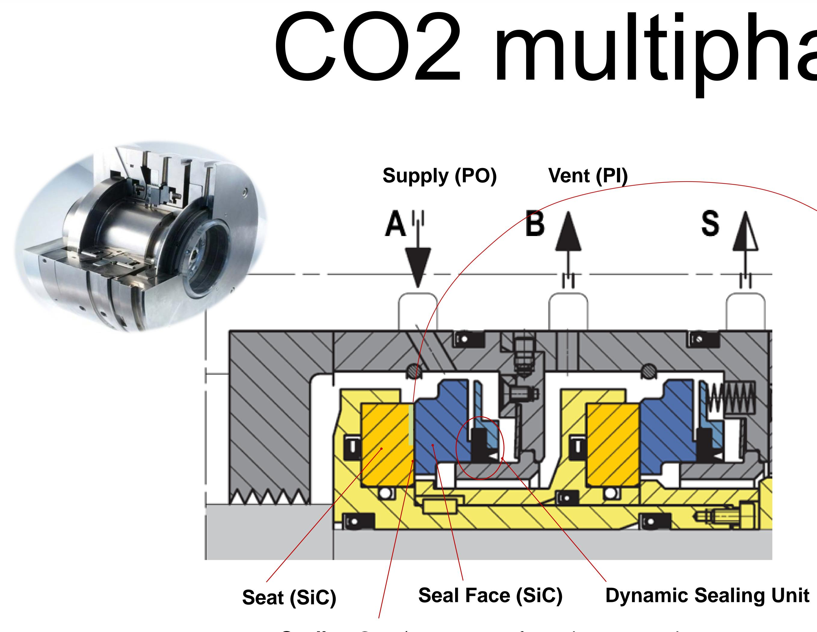
Sealing Gap (opens up to few micrometer when subjected to pressure and/or rotation)
