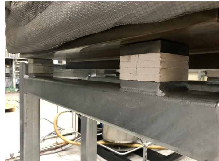
Recuperator Supports – insulated footing with polished stainless steel contact
