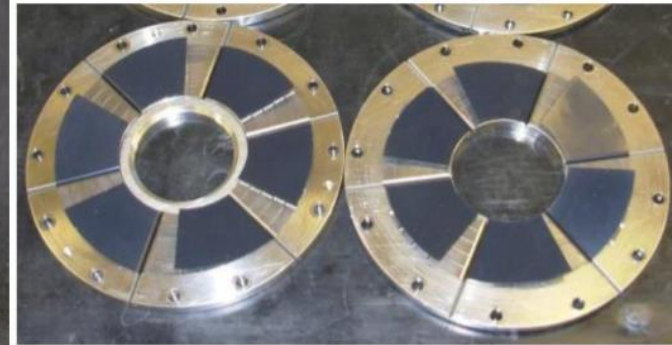
Gas Foil Journal (left) and Thrust (right) Bearings (Wright et al. , 2010)
