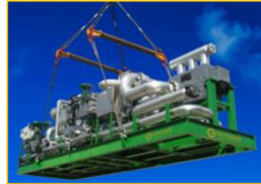
Heatric supply to Echogen EPS 100, the world's first commercial sCO 2 WHR unit
