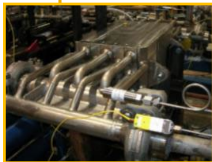
Heatric supply three PCHEs to Sandia National Laboratories sCO 2 Brayton test loop
