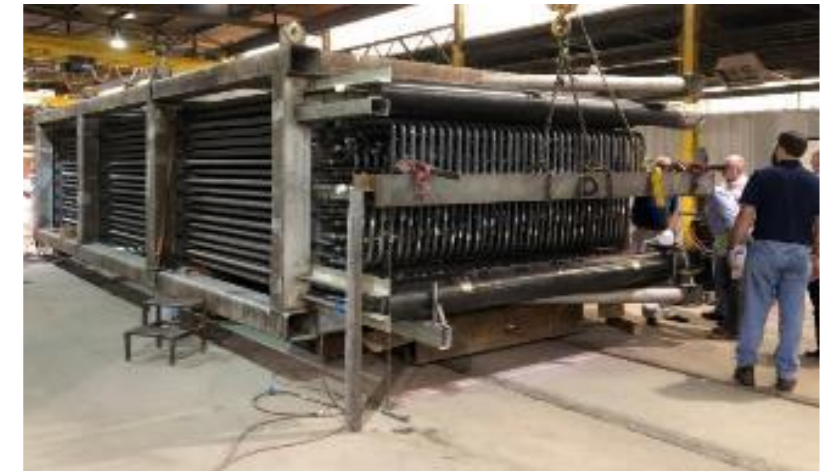
STEP 10 MWe Facility Natural Gas Fired Heater
