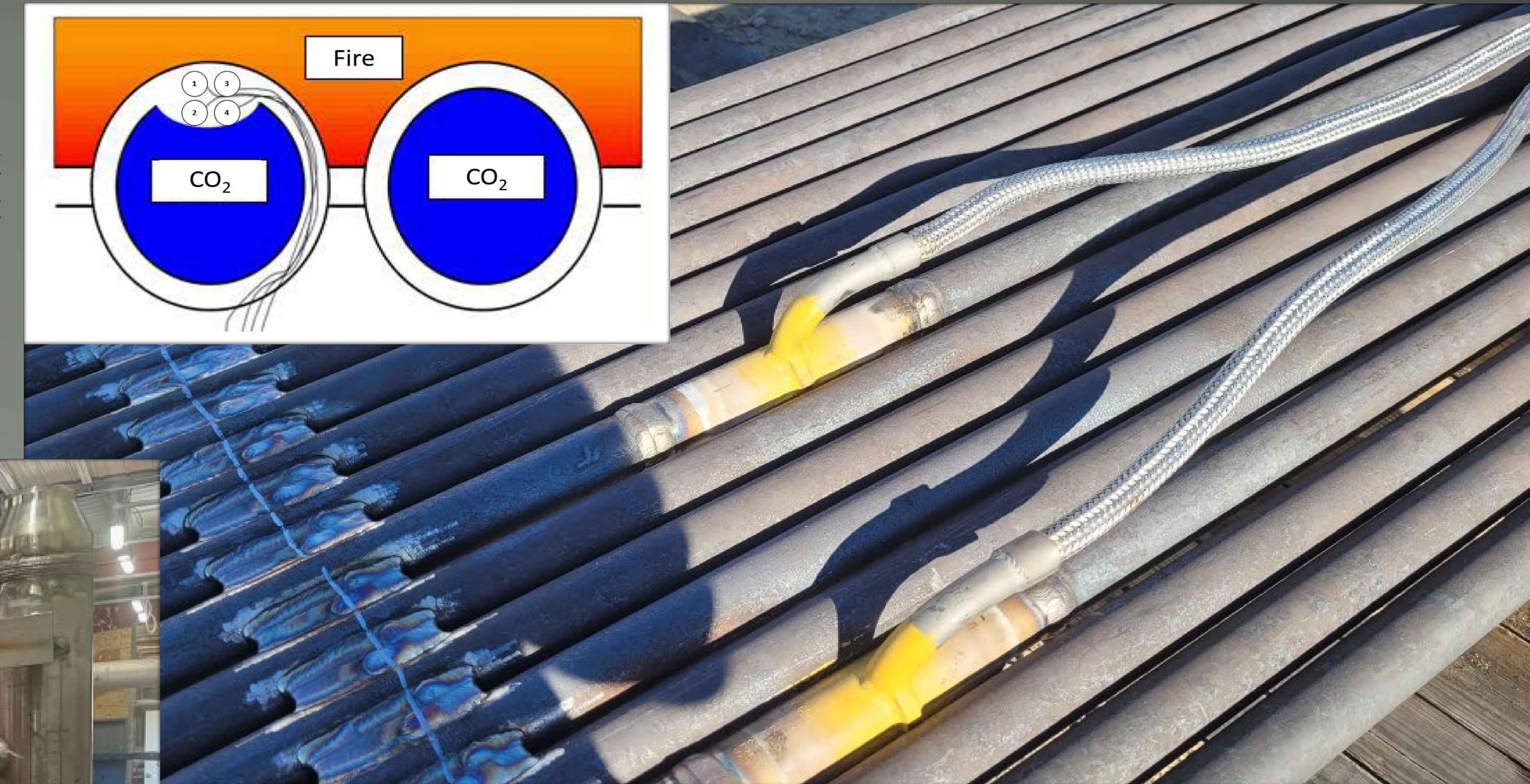
Fig13: Heat Flux Sensors Installed on PHX Piping.
