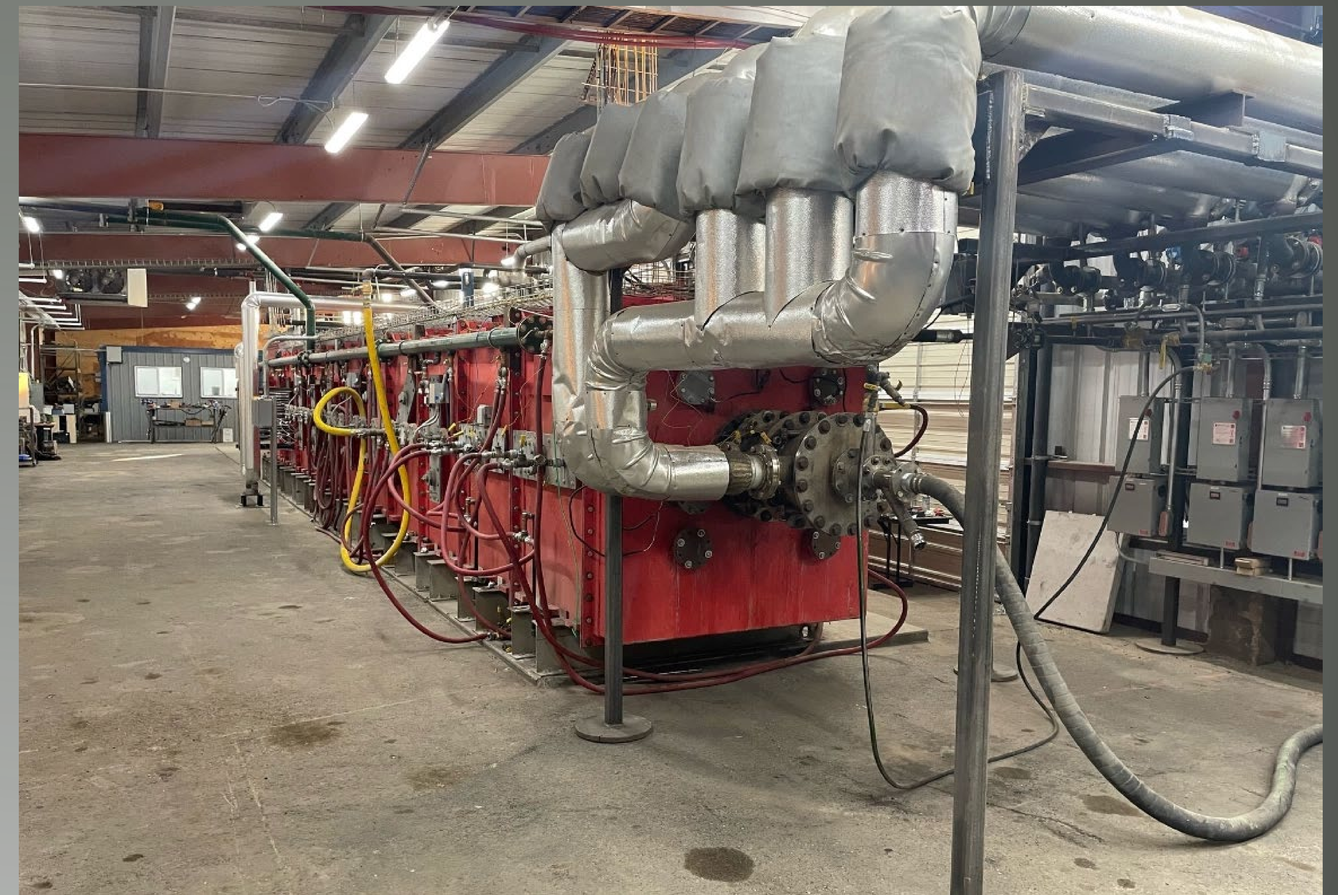
Fig2: L1500 Furnace Burner w/Inlet Fuel Manifold
