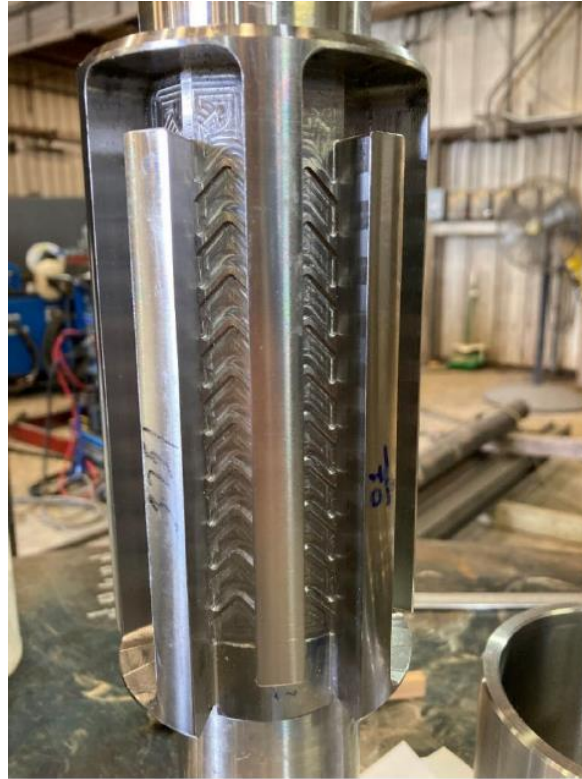
Figure 3. Machined flowpath for cooling flow featuring chevron ribs. At center is shown the terminating passage of the two symmetric, serpentine flowpaths.
