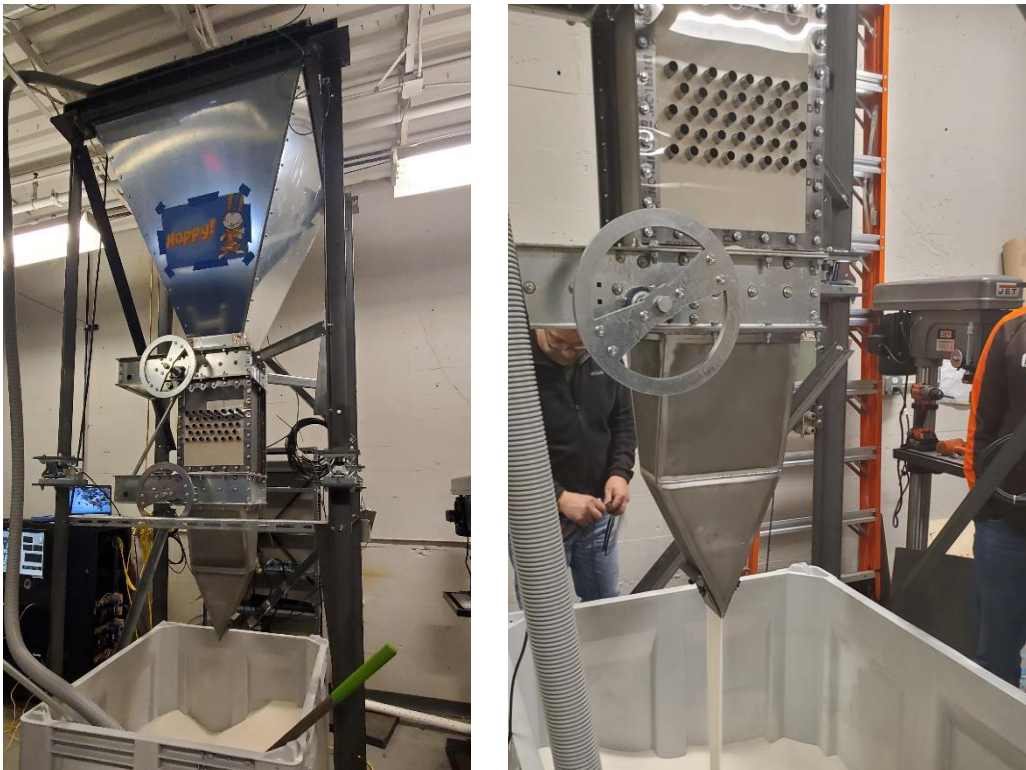
Figure 1: Echogen Moving Bed Heat Transfer test facility. In progress bare tube test shown at right.
