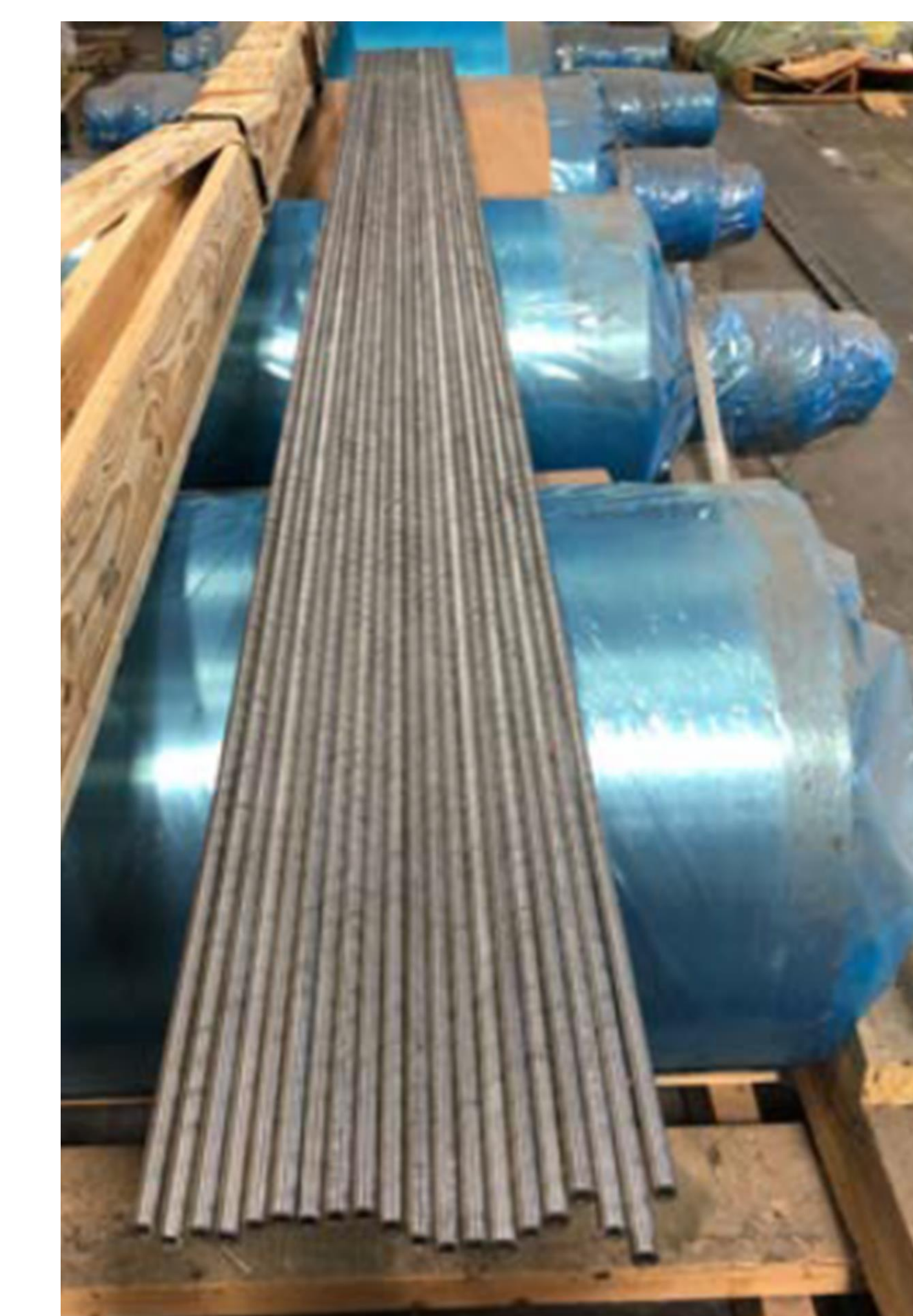
Welded and redrawn, 0.375" OD x 0.080" W
