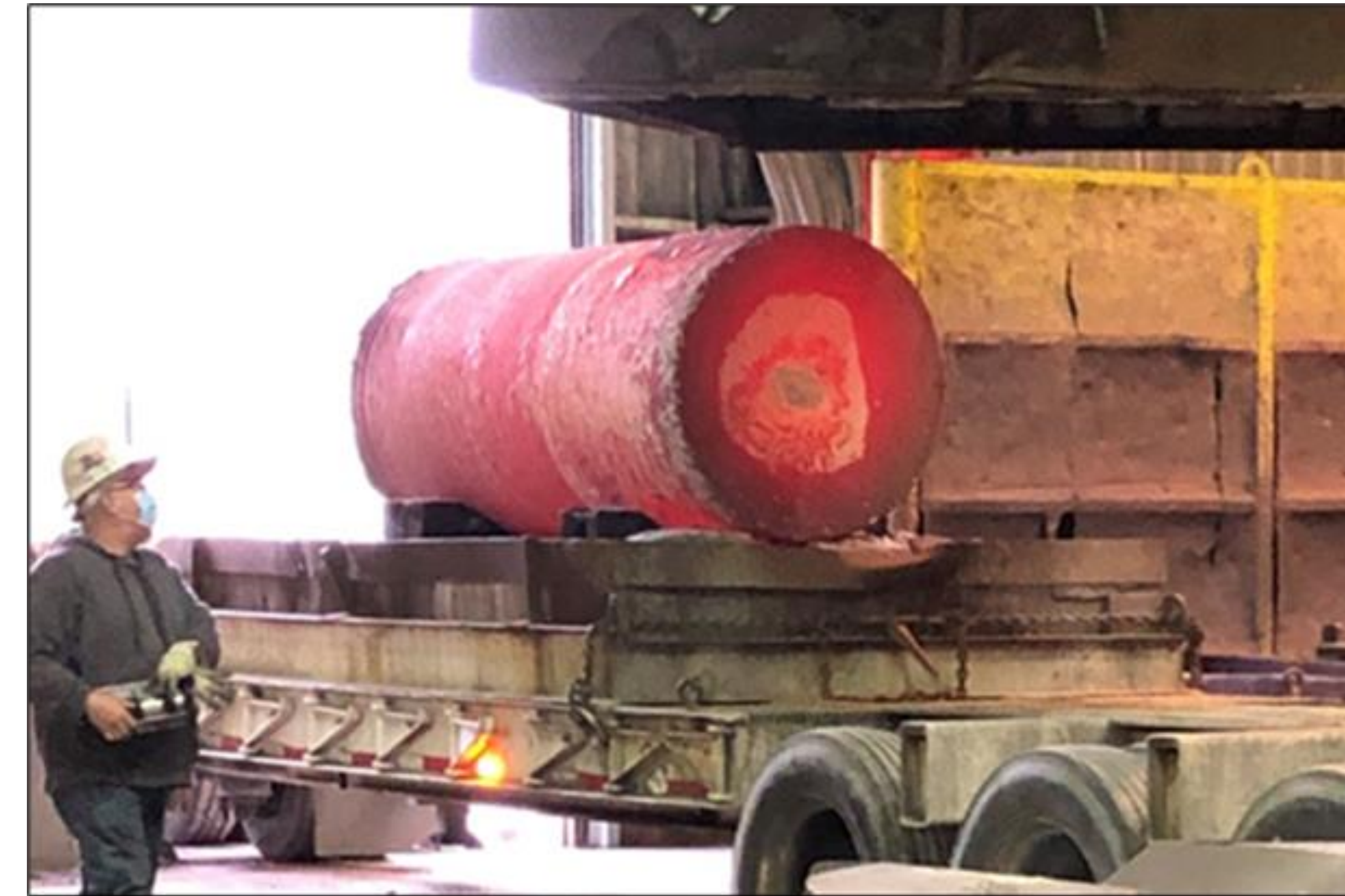
Largest 740H ingot produced by Special Metals in Huntington WV
