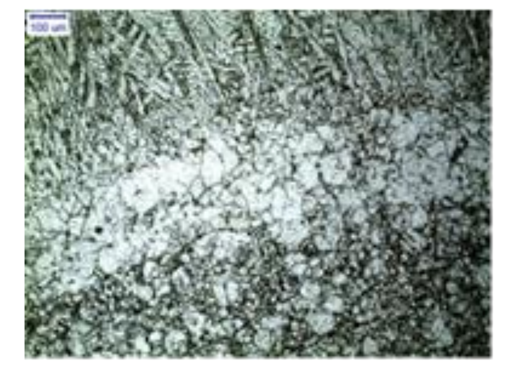
HIP 740H plate successfully welded to wrought 740H plate
