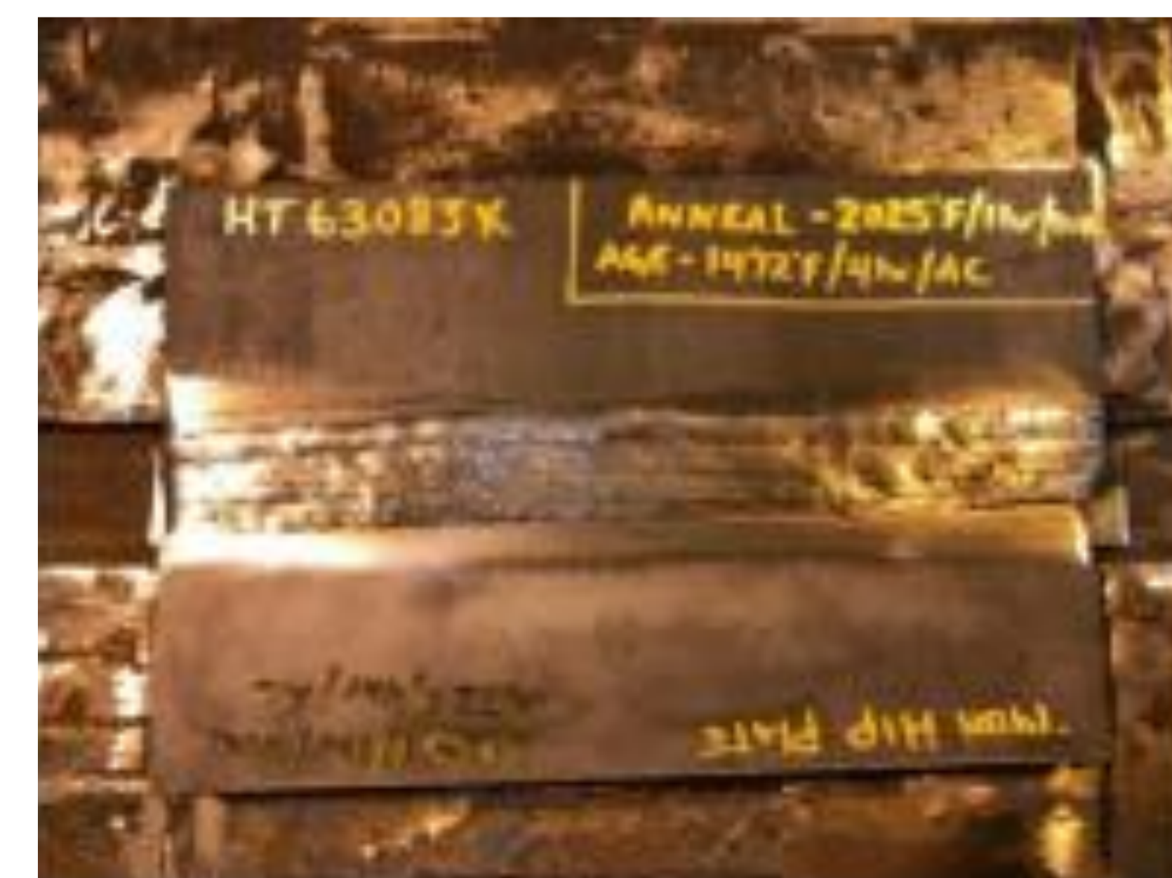
HIP 740H plate successfully welded to wrought 740H plate
