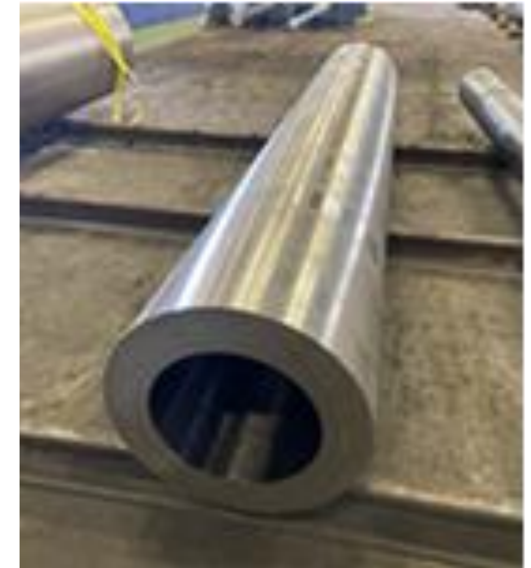
Extruded seamless pipe 22" OD x 3.7" W
