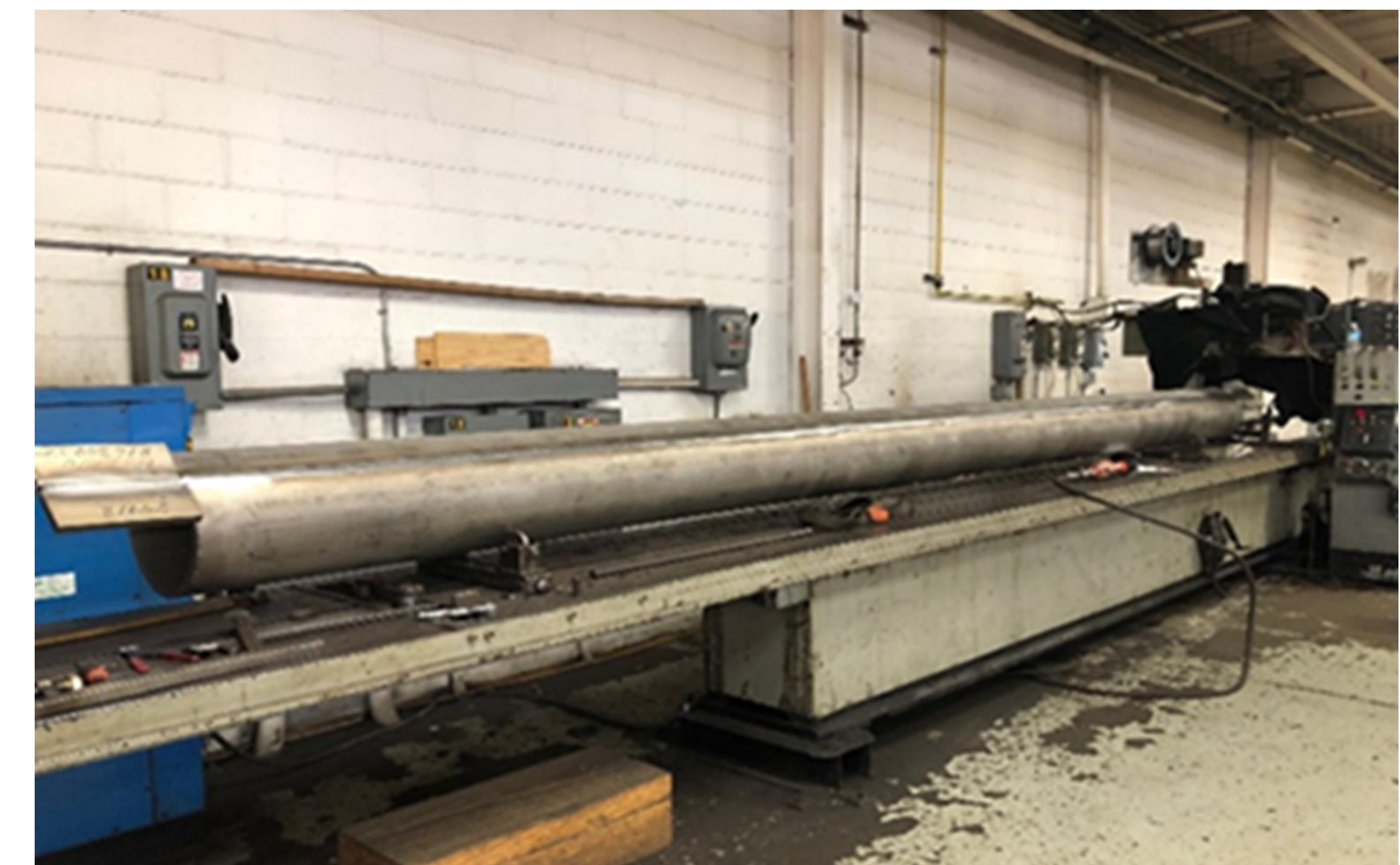
Welded pipe – 14" OD x 0.75" W x 20'
